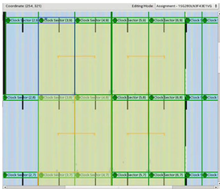
Figure 43. Clock Sector Boundary Layer in Chip Planner
